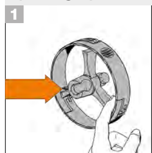
To open, raise the lug by hand or insert a screwdriver into the notch and open.
