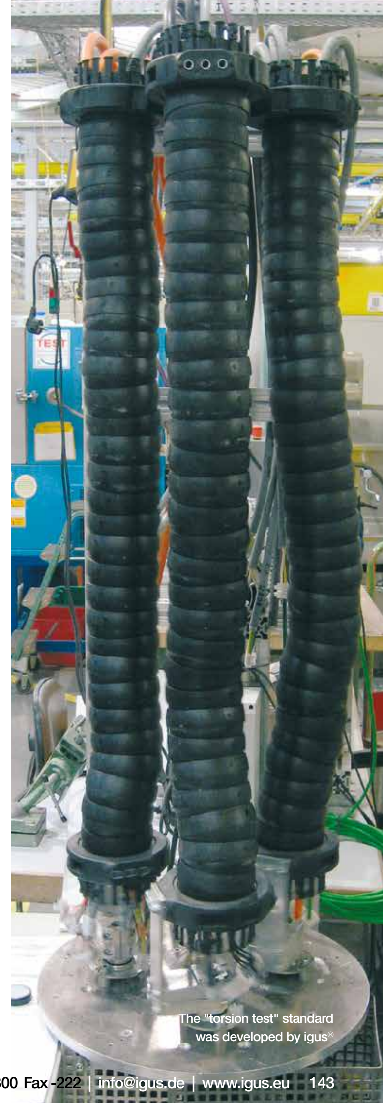
The CFROBOT shows absolutely no damage after more than 3 million movements
