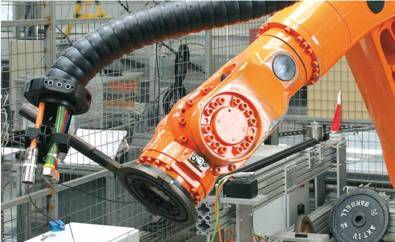
Individual strain relief for every cable allows easy replacement
