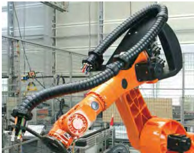
triflex® RS for a lean chain guide. Integrated spring rods generate directed pretension so that loops do not form in the working area
