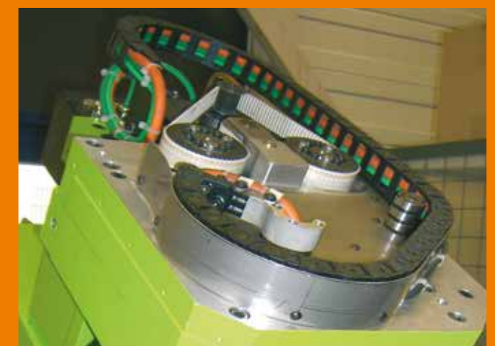
E2 mini, Series B15 - The motor spindle has a swivelling range of approx. 210^\circ
