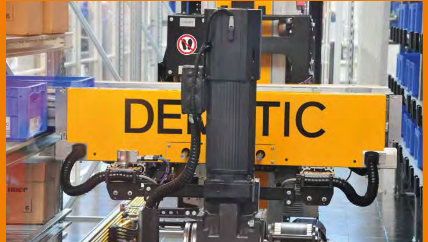
triflex® R in storage and retrieval system
