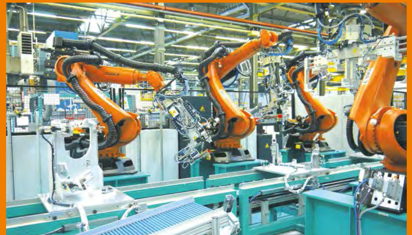
Flexible production - plant for the production of plastic vehicle tanks. In order to provide the end customer in the automotive industry with maximum flexibility, the production facilities are equipped completely with robots. The igus® RSP systems prevent loop formation of the e-chains® during the multi-axis movements of the robot.
